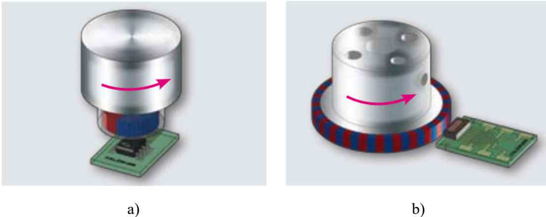
Figure 1.6 – a) Shaft-end mounting allows for absolute angular measurement, b) Circumferential mounting allows for incremental angular measurement [18].
