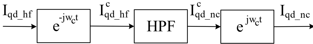
Figure A.51 – State block diagram of a carrier synchronous high-pass filter.
