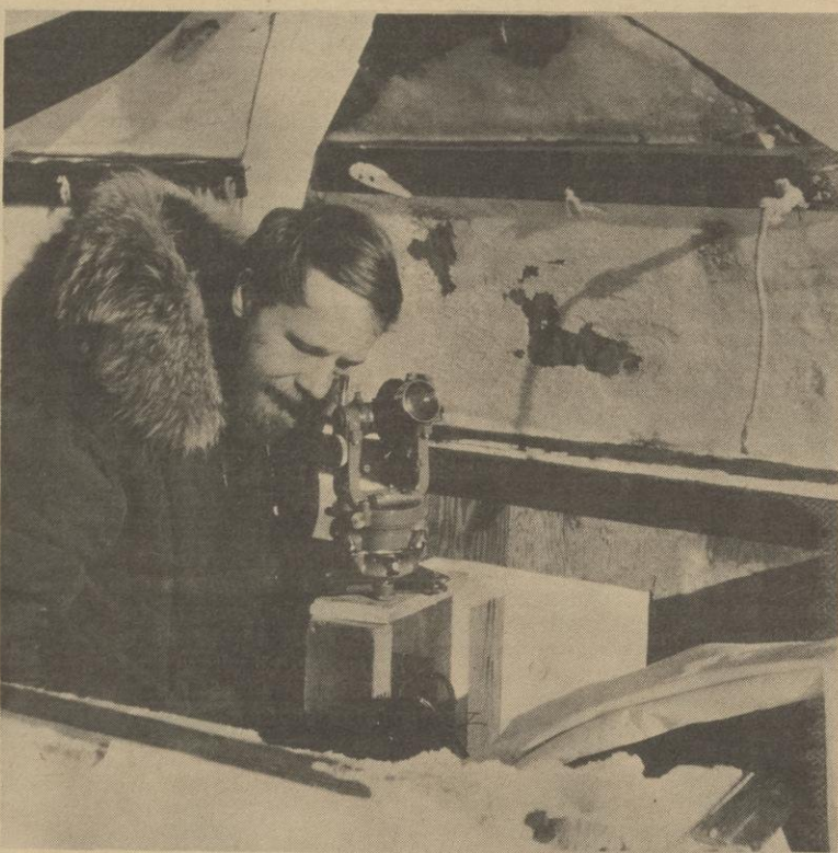
EXPLORER RECORDS COURSE —As Arlis II, the escaped ice island, travels southward in the Arctic Circle, Jim Pew peers through a theodolite, modern instrument for the time-honored sailor's way of learning a ship's navigational position by "shooting the stars."
