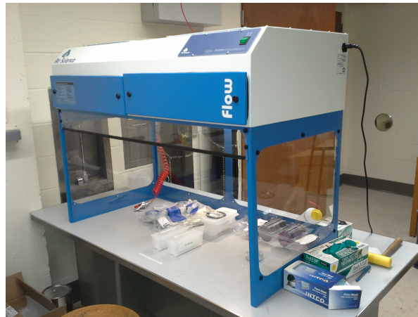
Figure 3.1: PURAIR Flow Hood in Lab
