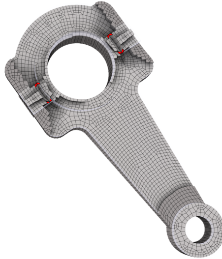
Figure 4.25: (a) Connecting rod mesh [103]; elements in red color are inverted. Some of the elements are penetrating.
