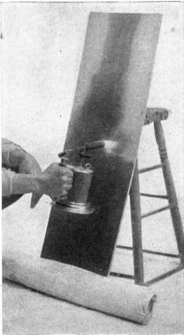
BURNING A CYPRESS BOARD WITH A GASOLINE TORCH: THE FIRST STEP IN THE SUGI PROCESS.
