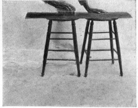
RUBBING THE BURNED CYPRESS BOARD WITH A WIRE BRUSH TO REMOVE THE CHARRED GRAIN, ACCORDING TO THE SUGI PROCESS.
