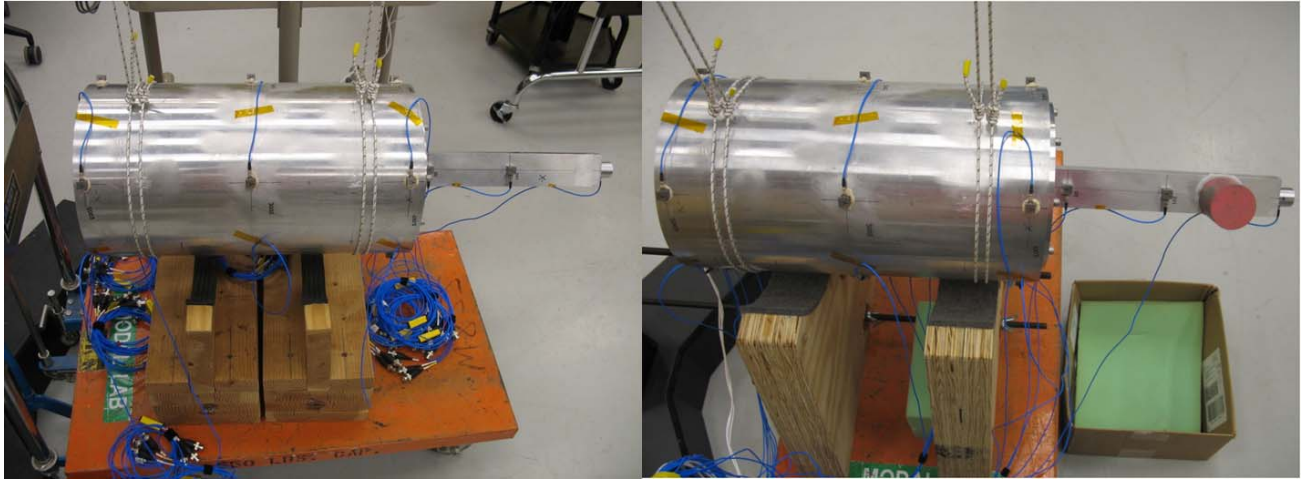
Figure 21. Cylinder-Plate-Beam System Experimental Set-up
