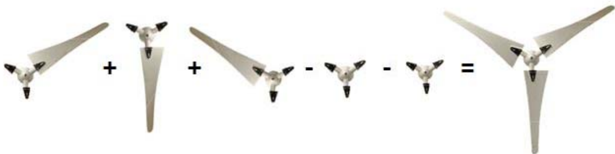
Figure 9. Transmission Simulator Ampair 600 Wind Turbine Substructuring Schematic
