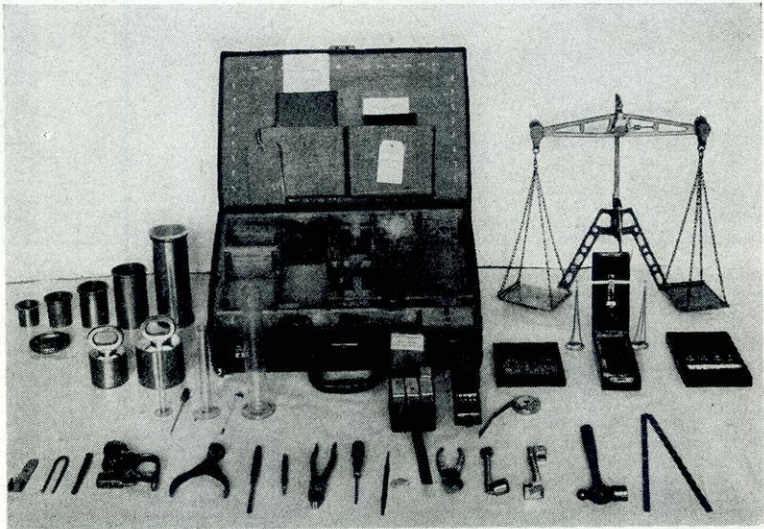
There are 85 pieces of standard equipment in this portable weights and measures kit used by state sealers in their work in war plants and other commercial institutions. In connection with this kit a large number of fifty pound weights and large sized measures are used.
