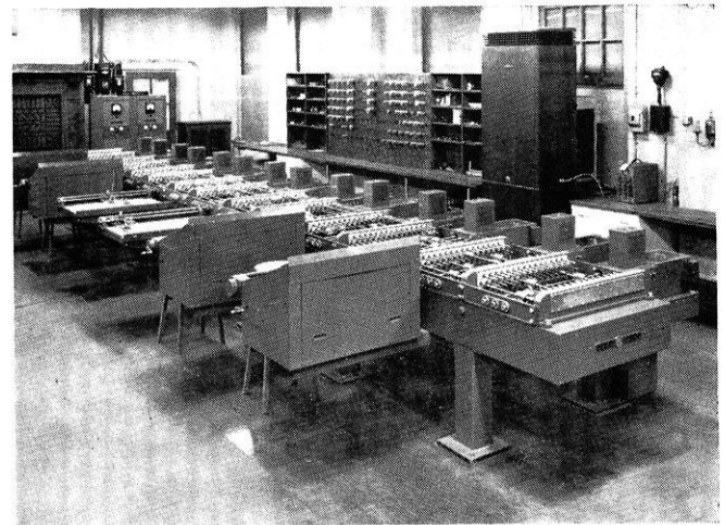
The differential analyzer applies to all problems that can be expressed by ordinary differential equations.
