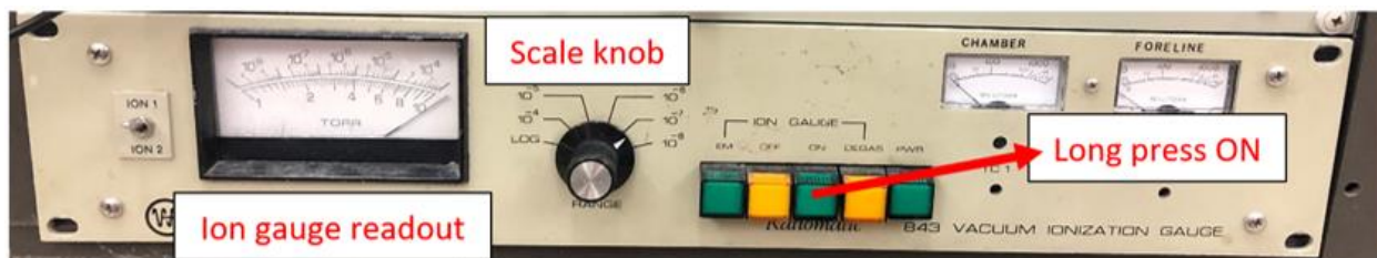
Figure 73: Picture shows the various parts making up 843 ionization gauge readout.
