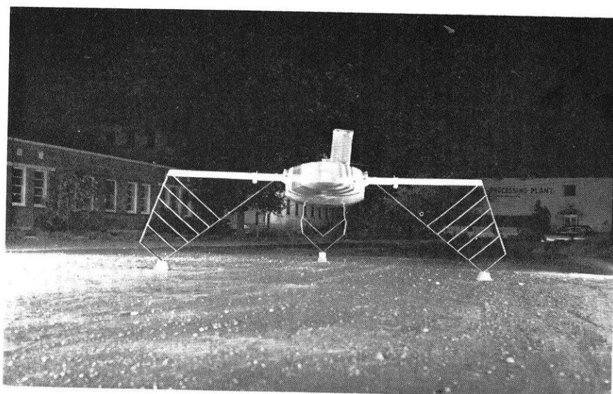
Figure 8.—Hydrofoil System of the Monitor
