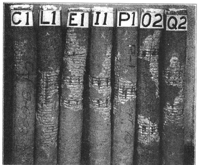
FIG. 3. Butt and lap splices after testing.
