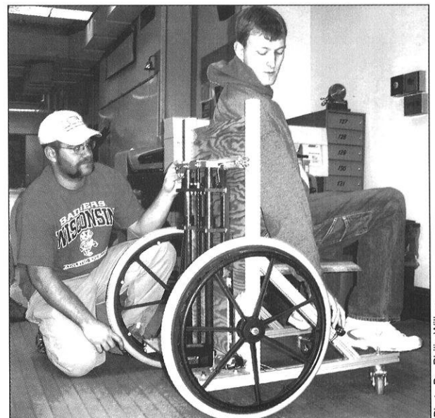
Students demonstrate the last prototype of a wheelchair that helps its user stand up.
