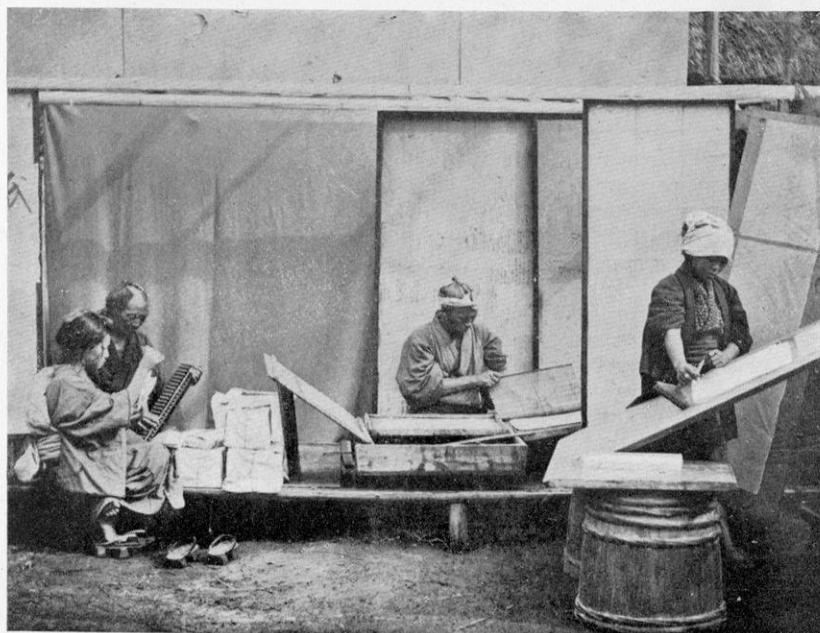
DIPPING PAPER SHEETS FROM THE PULP VAT AND DRYING
