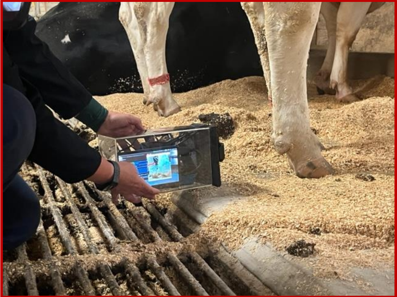
Figure 3.3 Real-time detection of DD on a portable, self-contained edge device in action.
