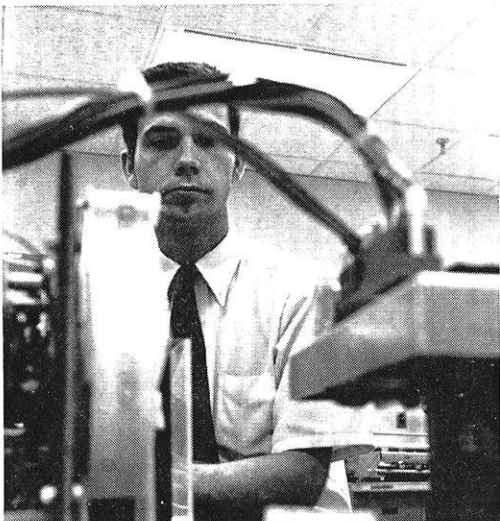
An engineer checks out a data collection machine using punched tape to record number and type of operations performed.
