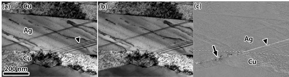
Figure 7.3.7 (a) and (b) Time resolved in situ straining of AgCu eutectic with 500 nm bi-layer thickness and incoherent twin interfaces and (c) difference image. Arrowheads mark stacking faults and the arrow marks displacement location of perfect dislocation slip in Cu. Interface in (c) is marked with the white dotted line.
