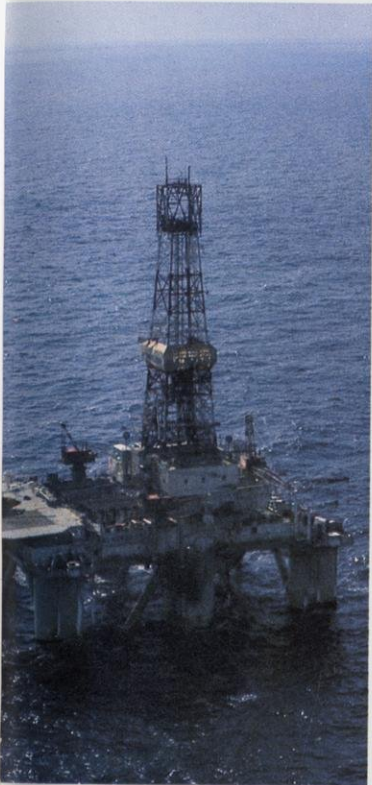
The self-propelled, semi-submersible rig Alaskan Star (left) has started exploratory drilling operations for Exxon on Georges Bank off the coast of Massachusetts. A gas separation plant at St. Fergus in northern Scotland (below) is scheduled for start-up in early 1982. It will process natural gas moved by subsea pipeline from fields in the North Sea in which Exxon has substantial interests. Dry gas will be sold to the British Gas Corporation. The separated liquids will undergo further processing to be sold as fuel and to provide feedstock for a major petrochemical plant in which Exxon has a 50 percent interest.
