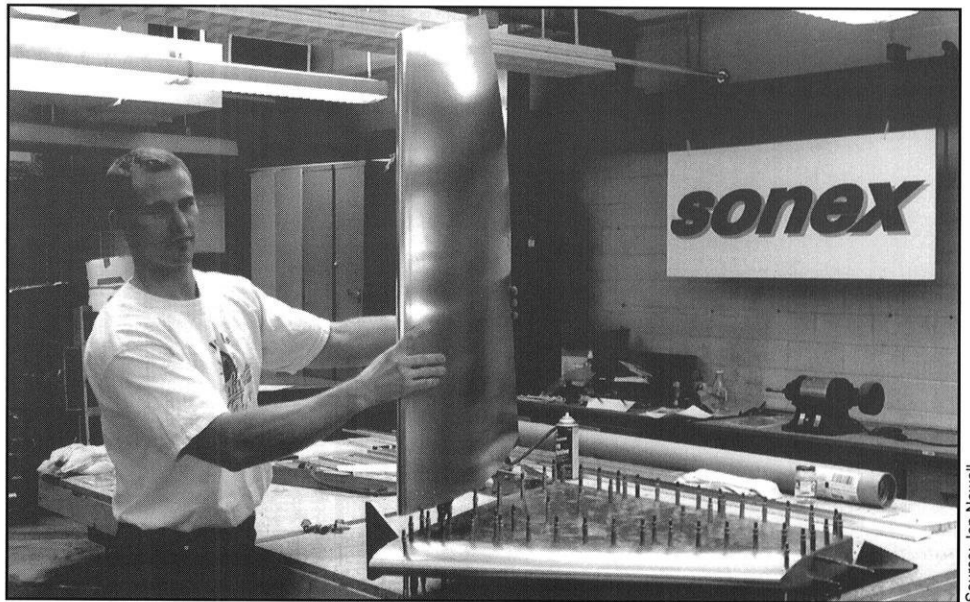
Project leader Mark Anderson holds the unfinished horizontal stabilizer next to the vertical stabilizer of the sonex plane
