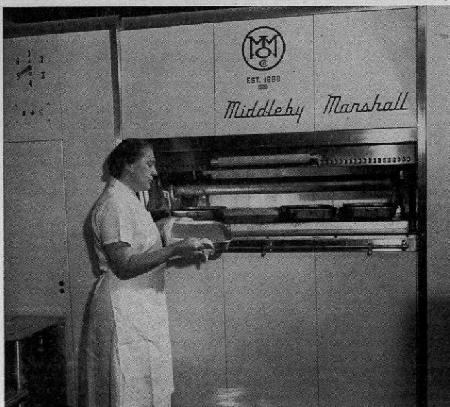
The rotary oven, with its six trays, works like a Ferris wheel. The Union kitchens make a number of special breads, pies, and sweet rolls, so the stand-up oven gets quite a workout each day.
