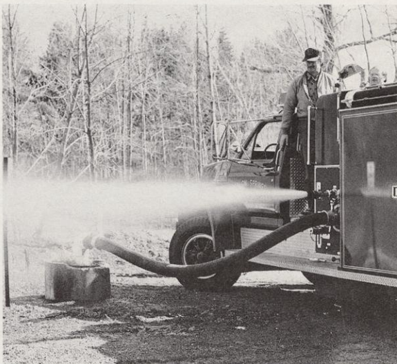
Testing a "dry" hydrant: a conduit from roadside to waterway in rural areas where pressurized hydrants are impractical.
