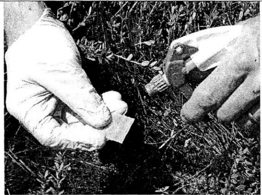
The membrane is cleaned with a spray of water.
