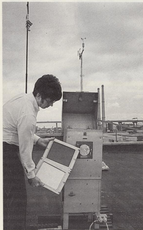
Contrast between a new and an exposed filter from a high volume air sampler in Milwaukee. Photo by Dean Tvedt
