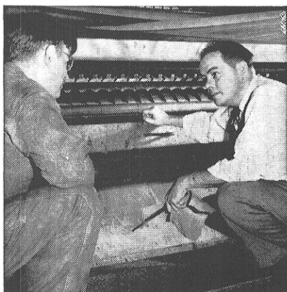
Edgar G. Boyce , Ashland State (right), helps a customer improve his method of applying silicate adhesive in the manufacture of corrugated boxboard.
