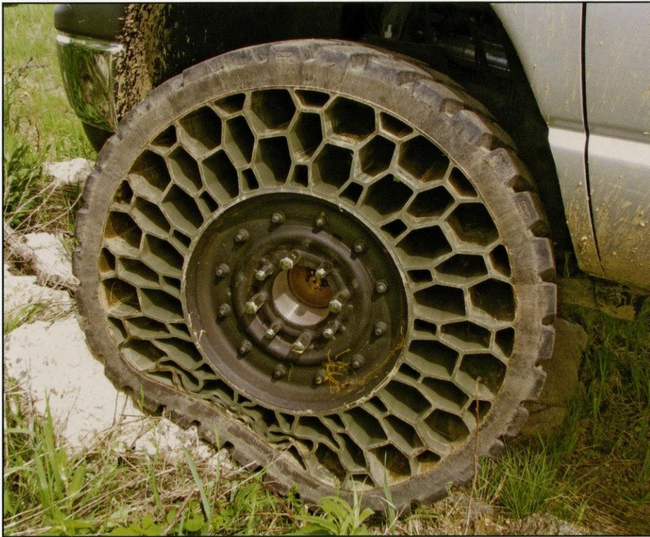
The design of the non-pneumatic tire enables military vehicles to easily maneuver through rough terrain.
