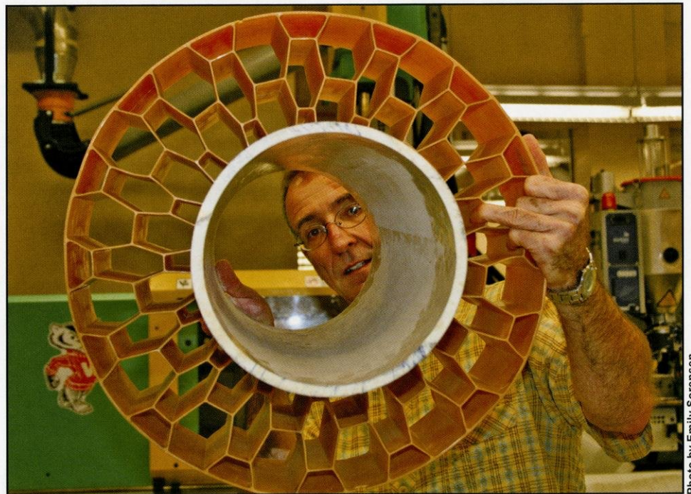
Professor Tim Osswald peers through the computer-optimized, honeycomb structure, which can be reconfigured for a variety of applications.
