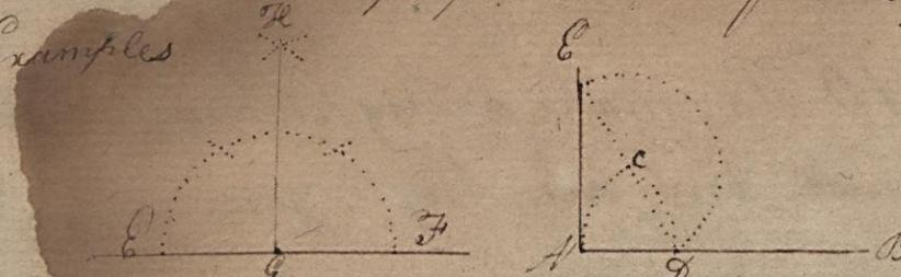
Problem 4. To let fall a perpendicular from a given point to a given line. Example.
