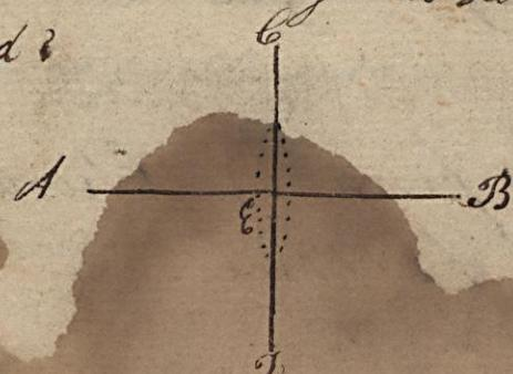
Problem 3. To erect a perpendicular from a point in a given line. Examples
