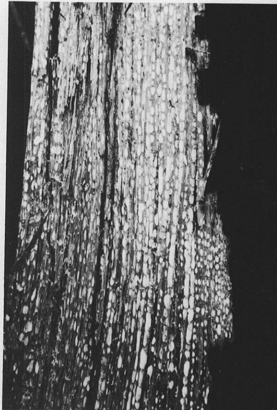
White pocket rot of oak. Most of the lignin in the white areas is degraded.
