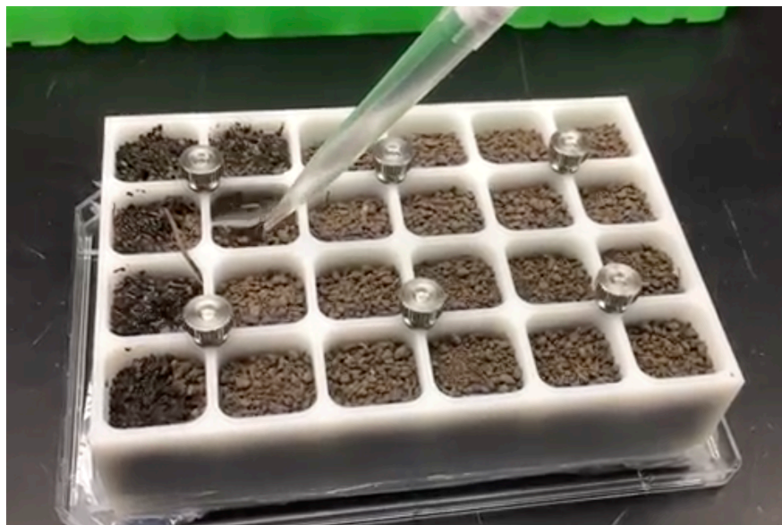
Figure 5.3: Applying water to assembled and loaded Type 1 “Deep-96” iplate device. This assembly can then be wrapped in parafilm or put in a cabinet or incubator.
