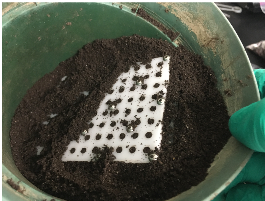
Figure 5.5: Type 2 Iplate assembled and buried in soil.
