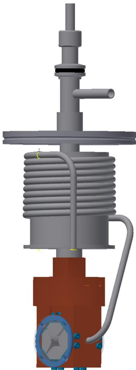
Figure 6.2 CAD figure of the new LN 2 cryostat for QTPI with copper tubing wrapped around the LN 2 reservoir.
