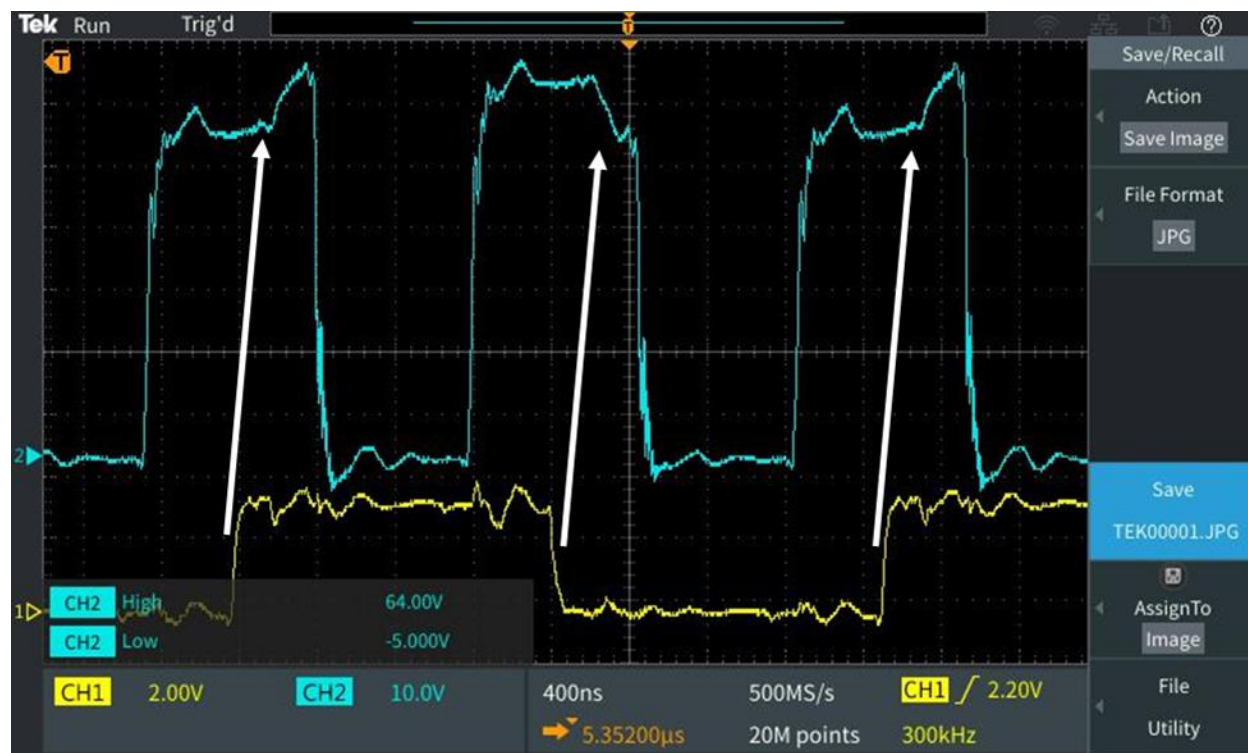
Figure 5.12 Oscilloscope traces of auxiliary waveform component (yellow) and final complex waveform (teal).
