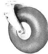
A Dowmetal yoke casting and tail wheel
