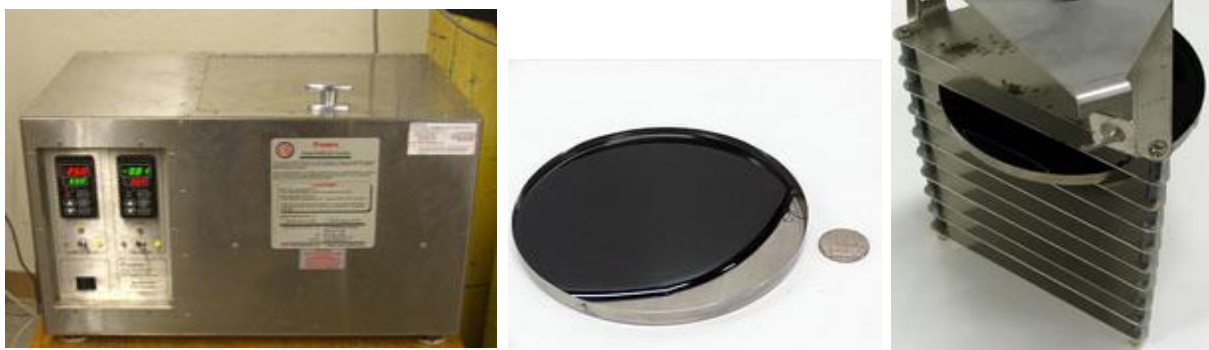
Figure III-2: (a) Pressure Aging Vessel (PAV); (b) PAV pan; and (c) PAV pan holder.
