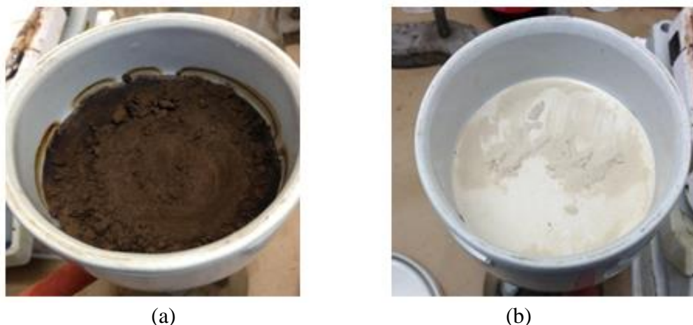
Figure III-3: (a) Asphaltenes + filler precipitated; (b) Mineral filler separated from asphaltenes.
