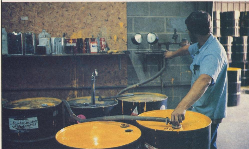
Testing barrels in a recycling plant to make sure they don't leak. Photo courtesy of Hydrite Chemical Company
