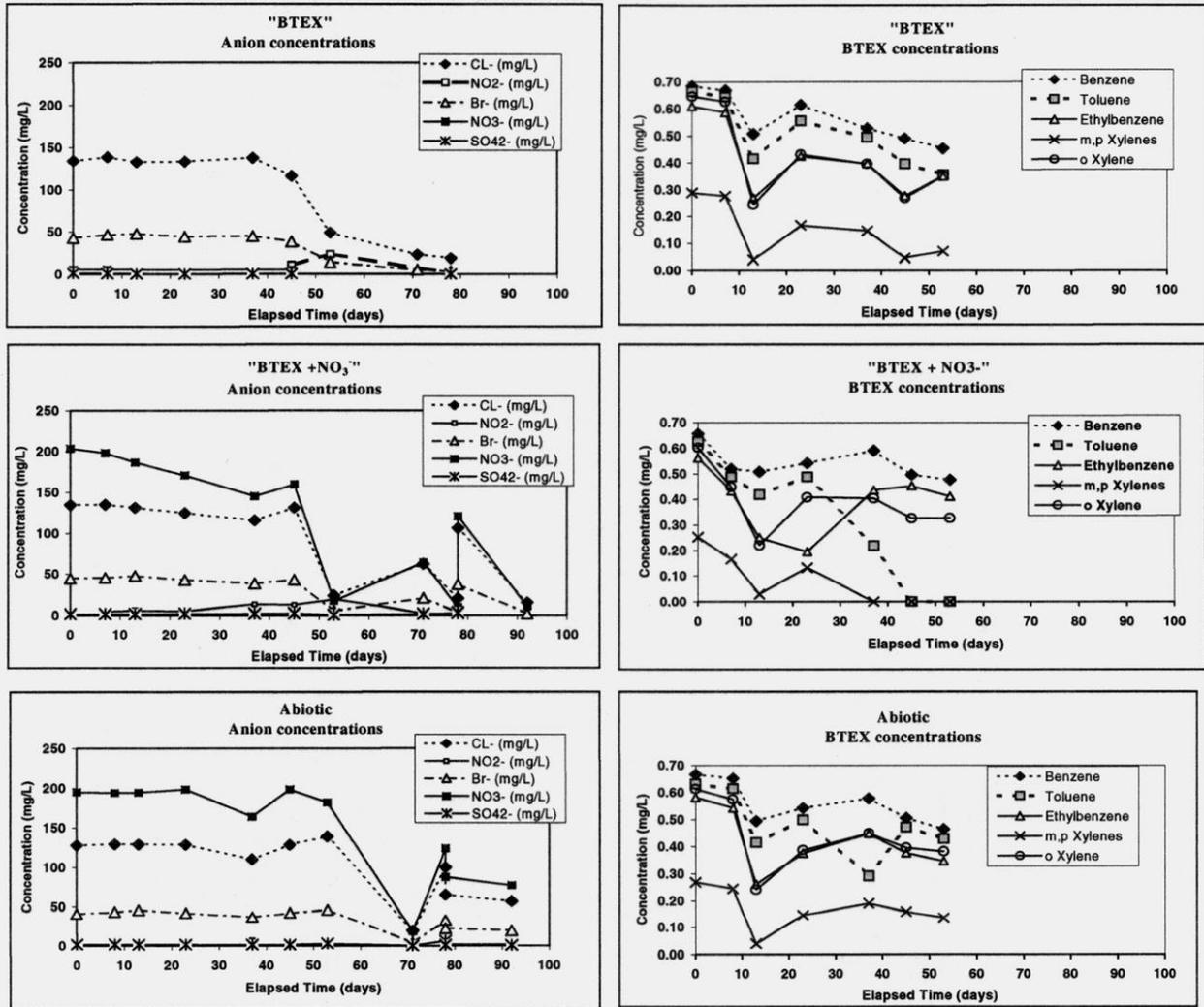
**Fig. 5.** Group 3 ISMs. Concentrations of BTEX and anions in ISMs located at Group 3. ISM was located between 5.5 to 7.5 feet below ground surface. The data used to construct these graphs are also available in Table 3.
