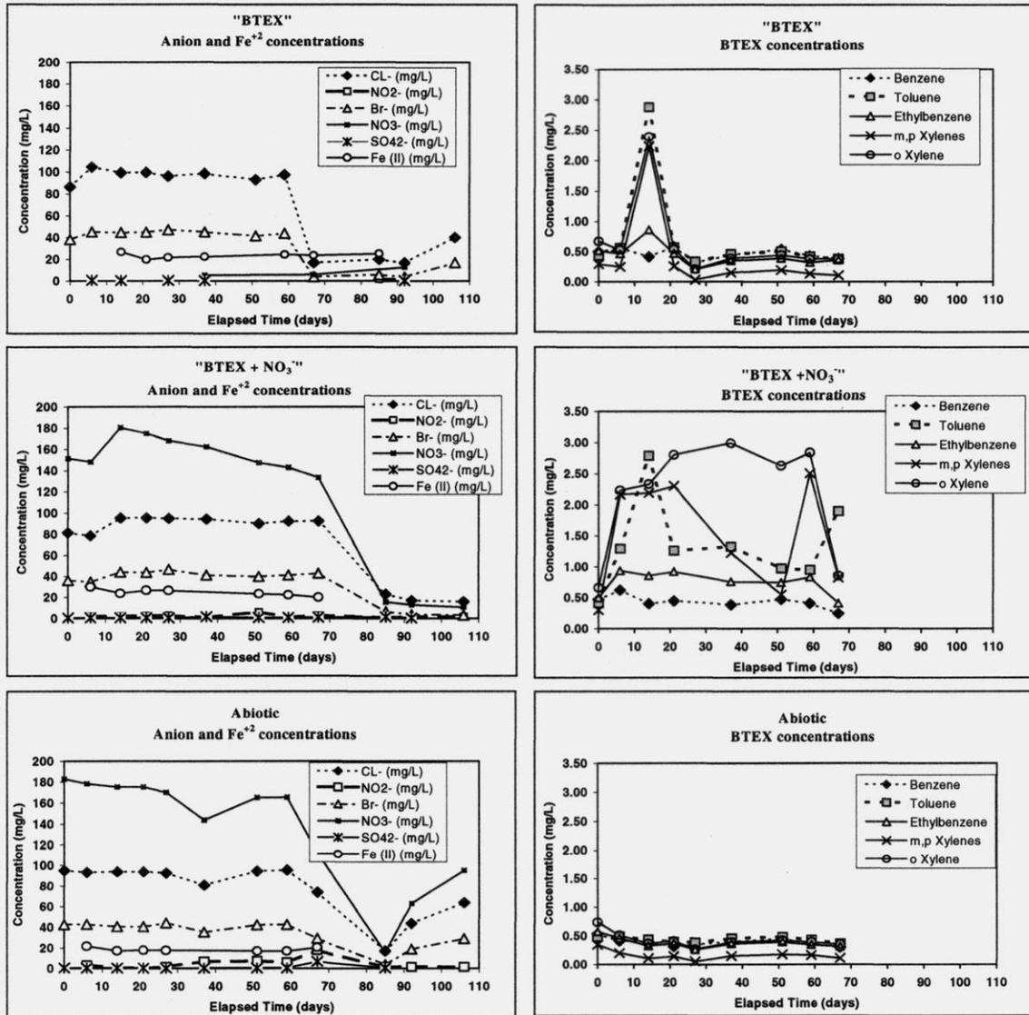
Fig. 3. Group 1 ISMs. Concentrations of BTEX, anions, and Fe<sup>+2</sup> in ISMs located at Group 1. ISM was located between 6 and 8 feet below ground surface. The data used to construct these graphs are also available in Table 1.
