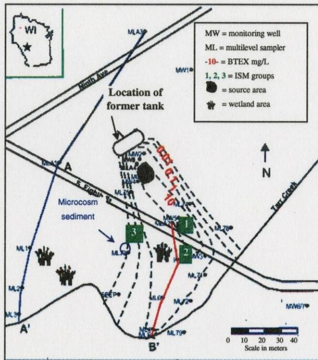
Fig. 1. Map of Fort McCoy, WI. BTEX concentrations for the plume are indicated by the dashed contours. The location of the microcosm sampling site and the locations of the ISMs are indicated. Section A-A' is the non-contaminated transect and section B-B' is the contaminated transect used for the tracer experiment.
