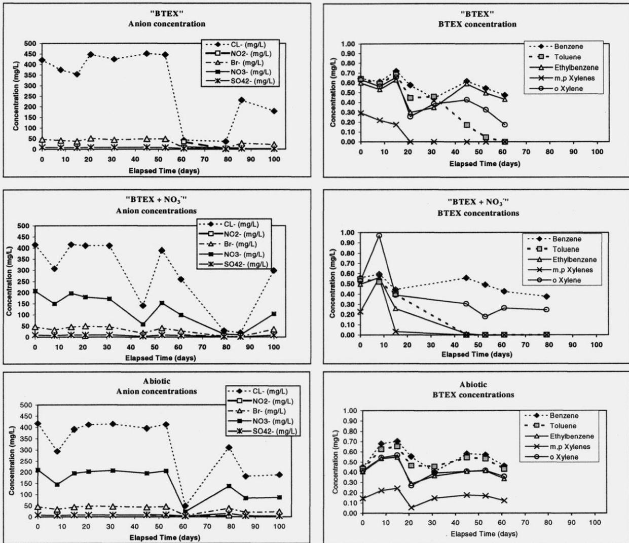
**Fig. 4.** Group 2 ISMs. Concentrations of BTEX and anions in ISMs located at Group 2. ISM was located between 5.5 to 7.5 feet below ground surface. The data used to construct these graphs are also available in Table 2.
