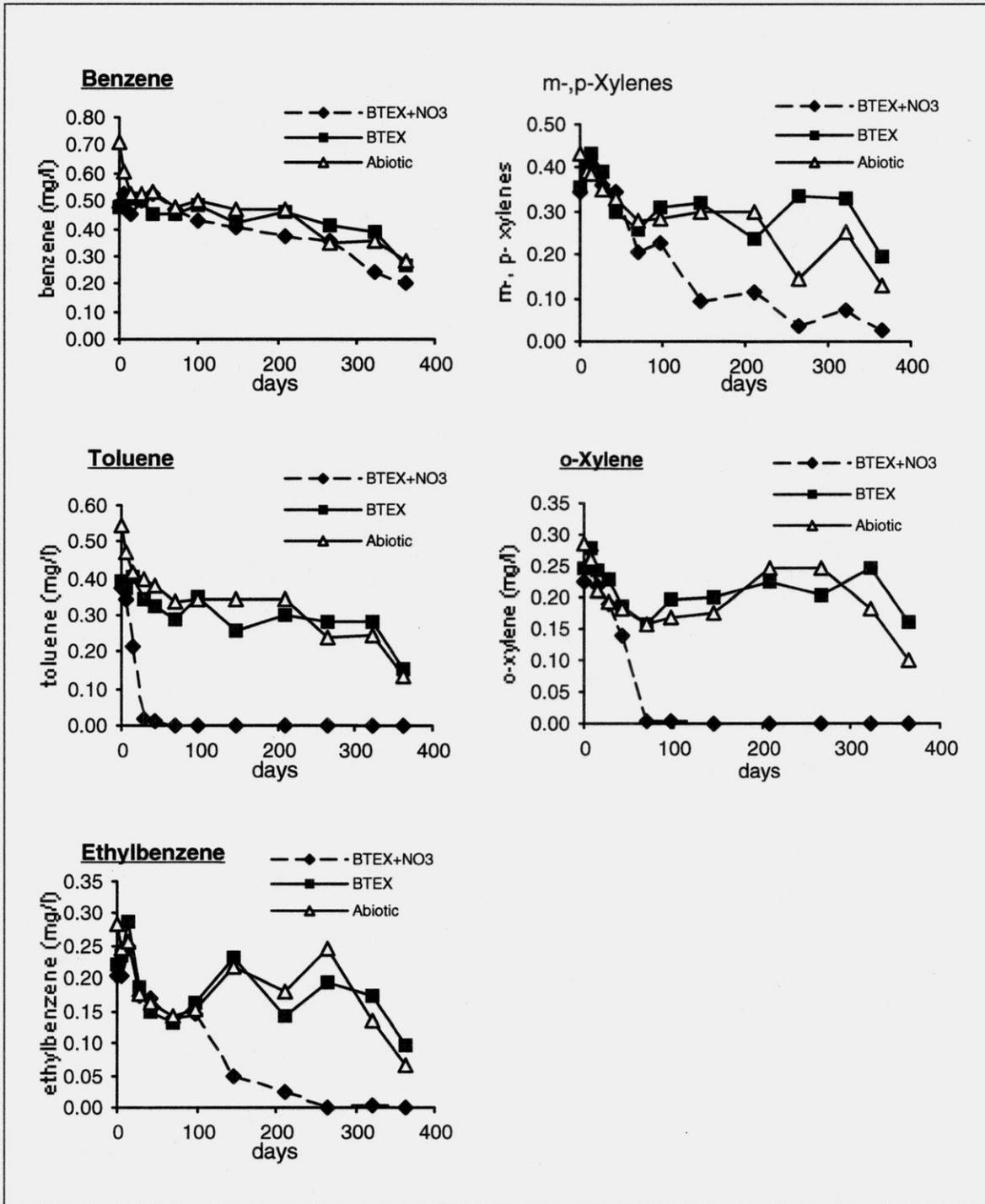
**Fig. 6.** Average benzene, toluene, *m*-&*p*-xylenes, and *o*-xylene concentrations measured in microcosms (with and without NO<sub>3</sub><sup>-</sup>) and abiotic controls. Error bars represent standard deviations of triplicate measurements.
