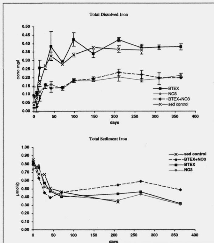
**Fig. 8** Average total dissolved and sediment Fe concentrations in microcosms. Abiotic controls were not analyzed for iron because of colorimetric interference. Error bars represent standard deviations of triplicate measurements.
