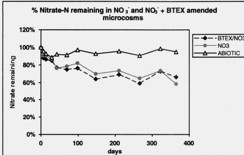
**Fig. 7** Average percent of  $\text{NO}_3^-$  remaining in microcosms amended with  $\text{NO}_3^-$ , with and without BTEX.
