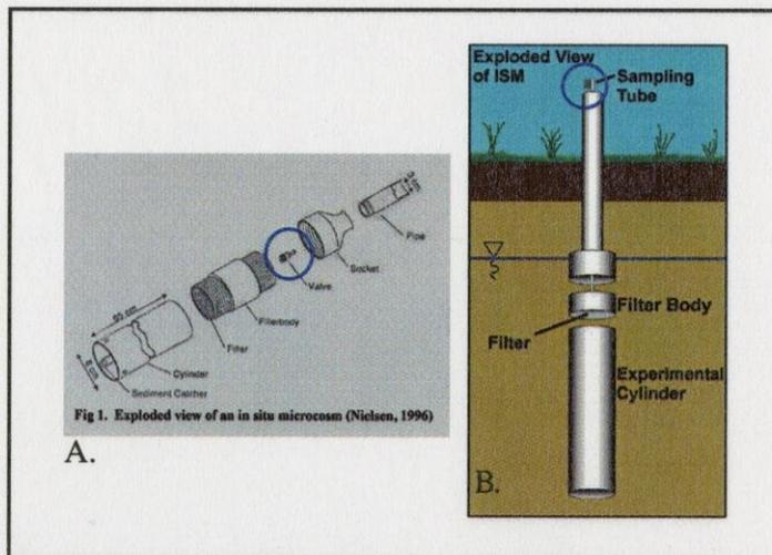
Fig. 2. Design of *in situ* microcosms. Panel A. Main ISM components in the original design. The valve is within the ISM itself. Panel B. Diagram of the ISM components in the improved design. The sampling valve is now at the top of the sampling tube, above the ground surface.
