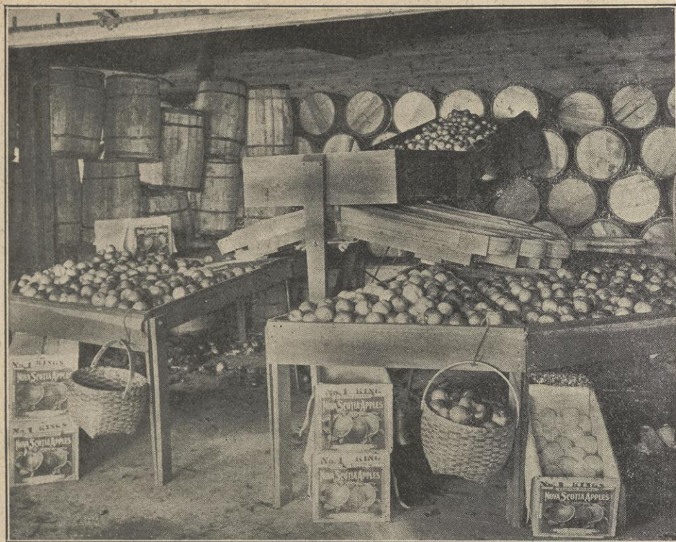
A simple apple-grading machine, as used in the fruit warehouse at Waterville, N.S.
