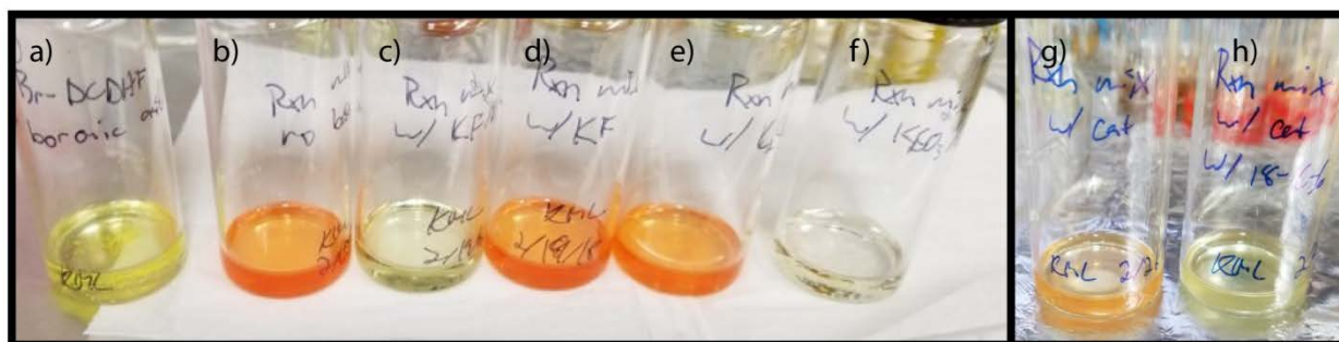
Figure 29: Reaction mixtures with various types of bases. All contain 4 mM each of 7 and 8 b)-h) contain 100 μM catalyst, a) no catalyst, no base b) no base c) KF, 18-C-6, d) KF, no 18-C-6, e) K 2 CO 3 , no 18-C-6, f) K 2 CO 3 , 18-C-6. g) no KF and no 18-C-6, h) no KF and with 18-C-6.
