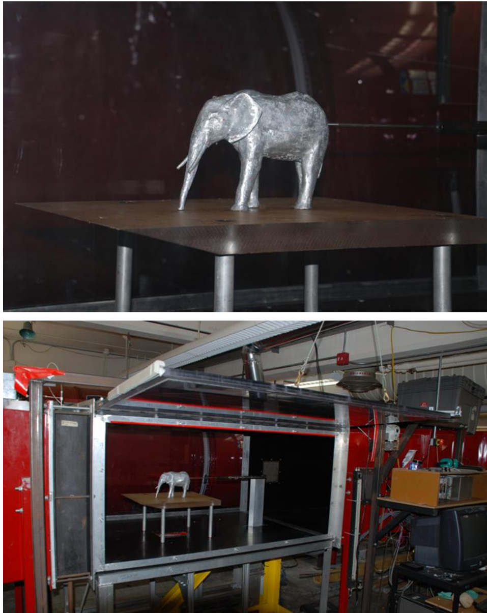
Fig.1. (Top) The solid aluminum elephant casting connected to a sting balance and placed on four ball bearings in recessed cavities in a solid Plexiglas sheet with a knife edge front end. (Bottom) The 4.8 cm thick Plexiglas sheet mounted on four posts bolted to the floor of the recirculating wind tunnel with a 0.9 x 1.2 x 1.84 m working section.
