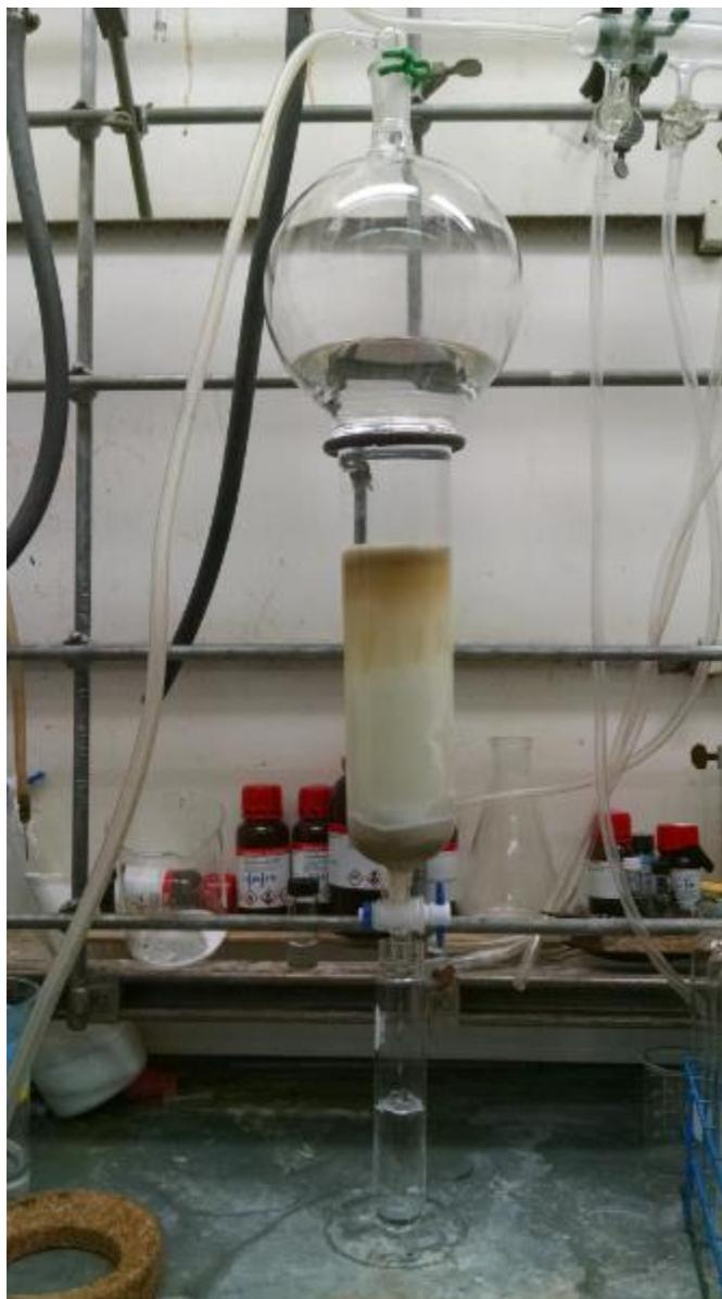
A replicate of the flash column utilized for removal of (*S*)-(-)-alpha-methylbenzylamine from the product amine diastereomeric mixture, during the separation. 150 mL fractions were taken.
