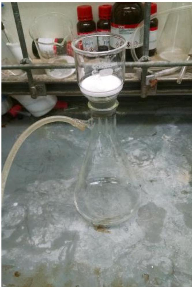
Fritted filter used for filtration of HCl salt from diethyl ether:dioxane solution, equipped to an Erlenmeyer flask, connected to a vacuum aspirator. Use of a clamp to secure the flask is recommended.
