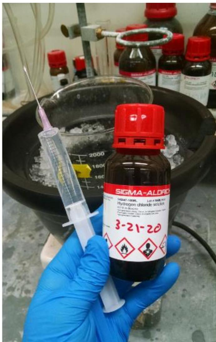
0.1 M solution of **4** + **diastereomers** from column in 0° C, diethyl ether, on stir plate (background), and syringe of 4 M HCl solution in dioxane to be added dropwise (foreground).
