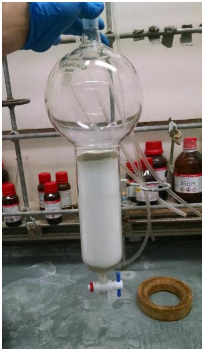
Flash column packed with silica utilized for removal of (*S*)-(-)- $\alpha$ -methylbenzylamine from the product amine diastereomeric mixture.
