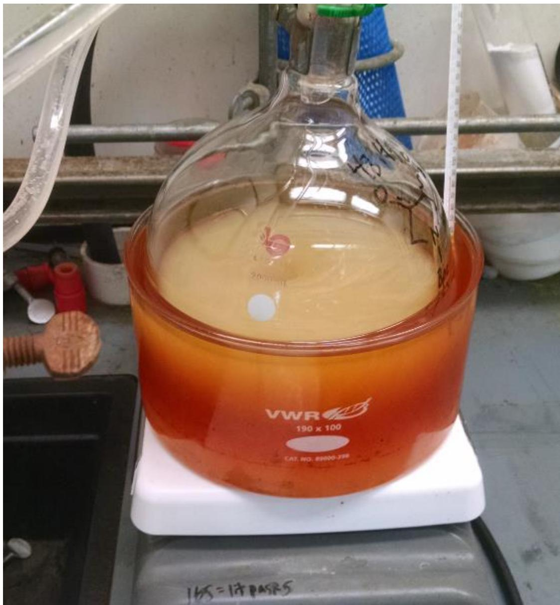
Light yellow reaction mixture after heating reaction mixture with sodium cyanoborohydride for 15 hours at 75° C.
