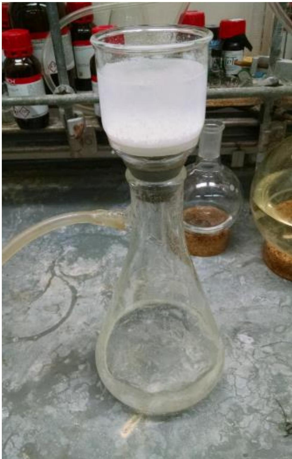
Vacuum filtration of the precipitated **APC**. Use of a clamp to secure the flask is recommended.
