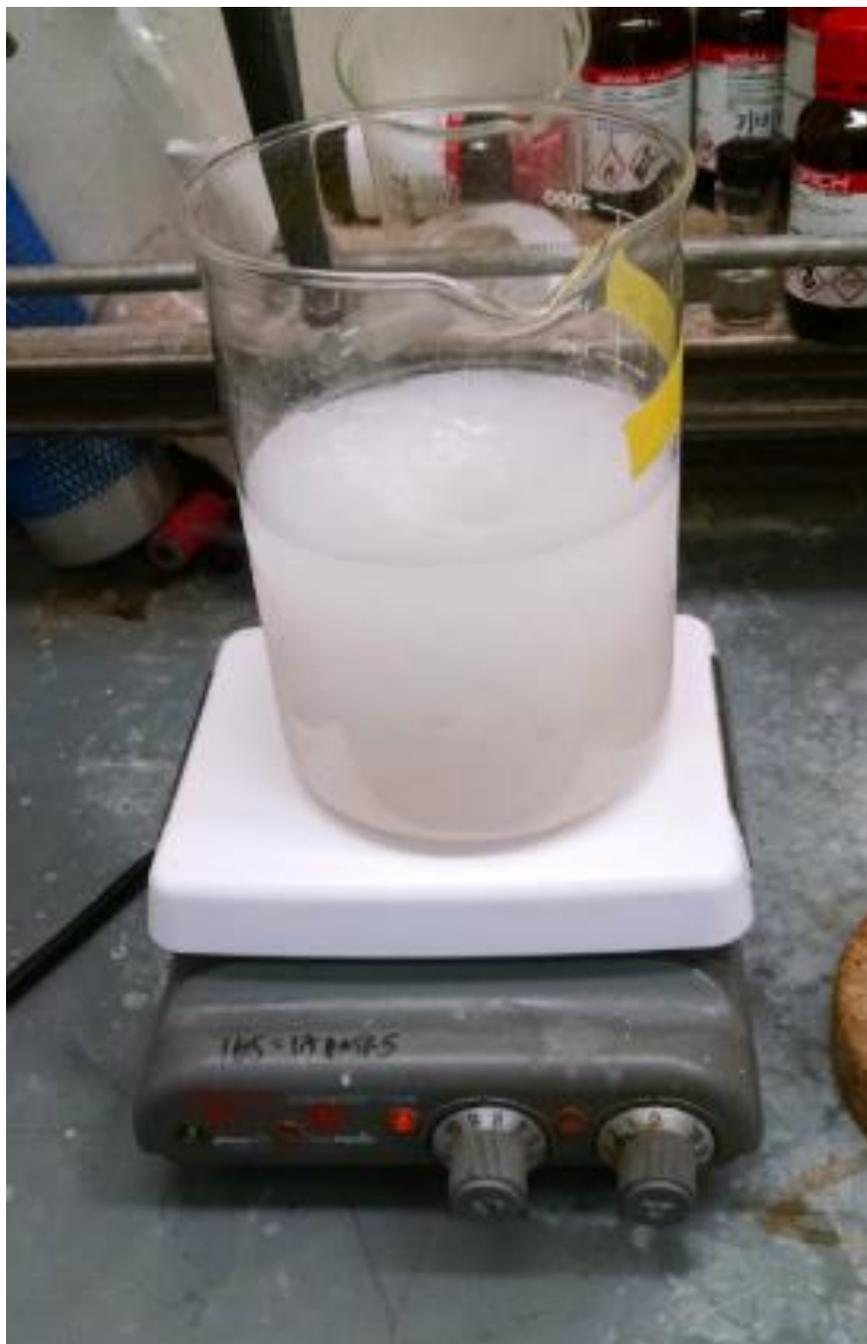
After complete addition of the ethyl acetate layer containing crude **APC**, a white/tan precipitate appears.
