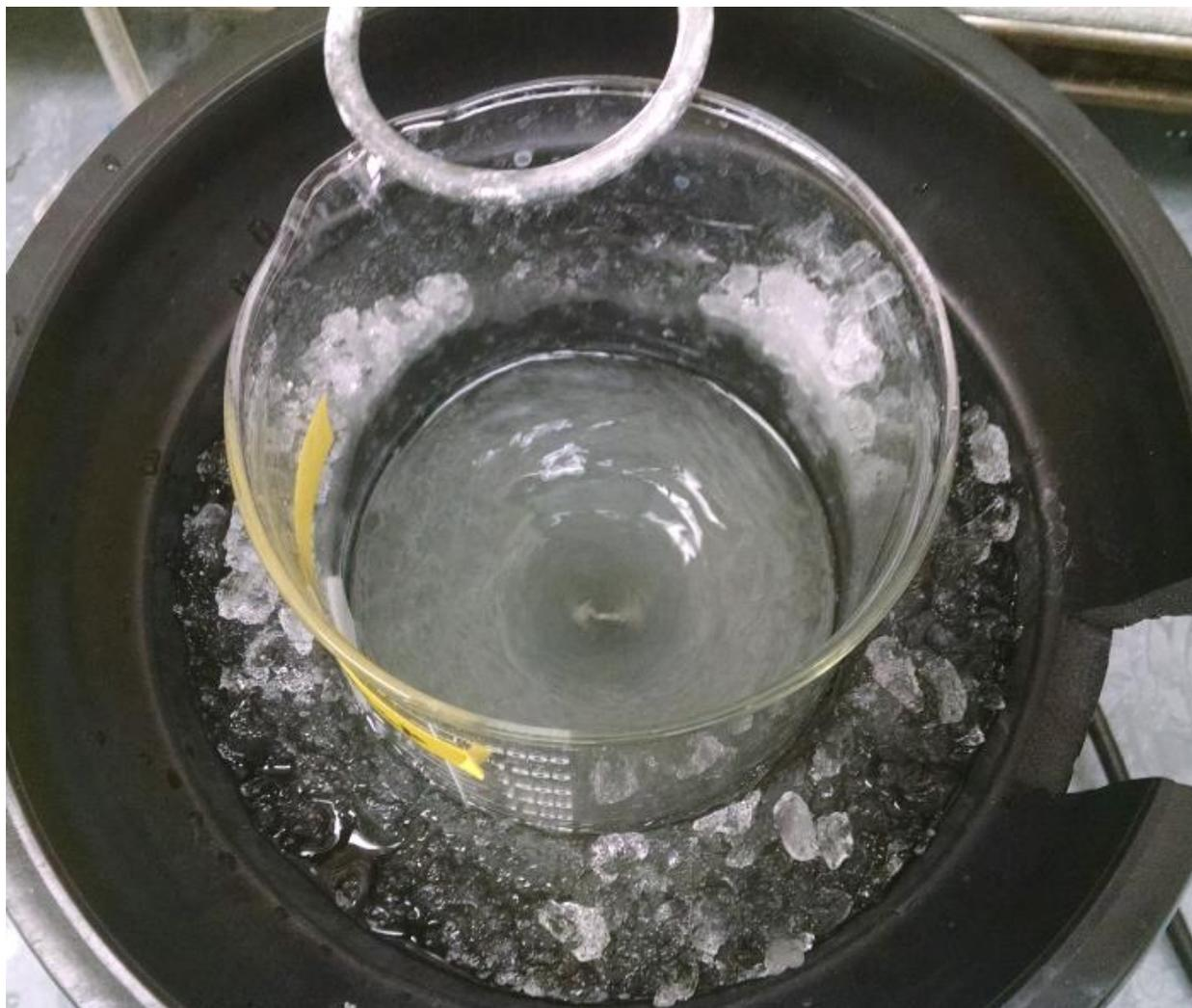
Initial formation of HCl salt during ten-minute period after about 10 % of 4 M HCl dioxane solution has been added. The cloudy slurry often takes ten minutes to form after initial addition of the first 10 % of 4 M HCl dioxane solution.
