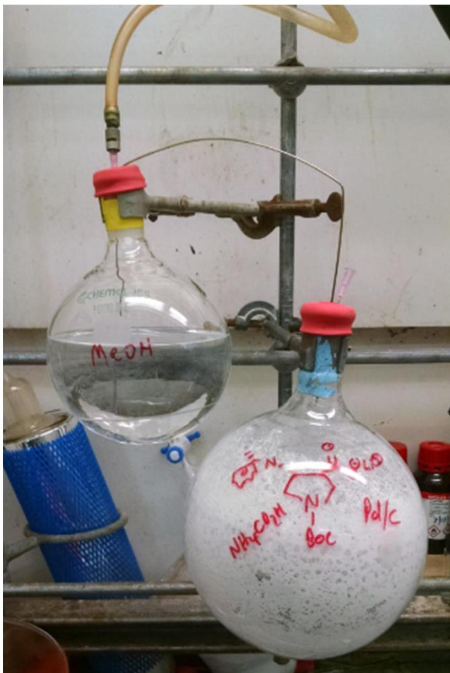
Crude saponification product **5**, ammonium formate, and Pd/C in a 2 L round bottom equipped with a stir bar, with MeOH being transferred in via cannula.
