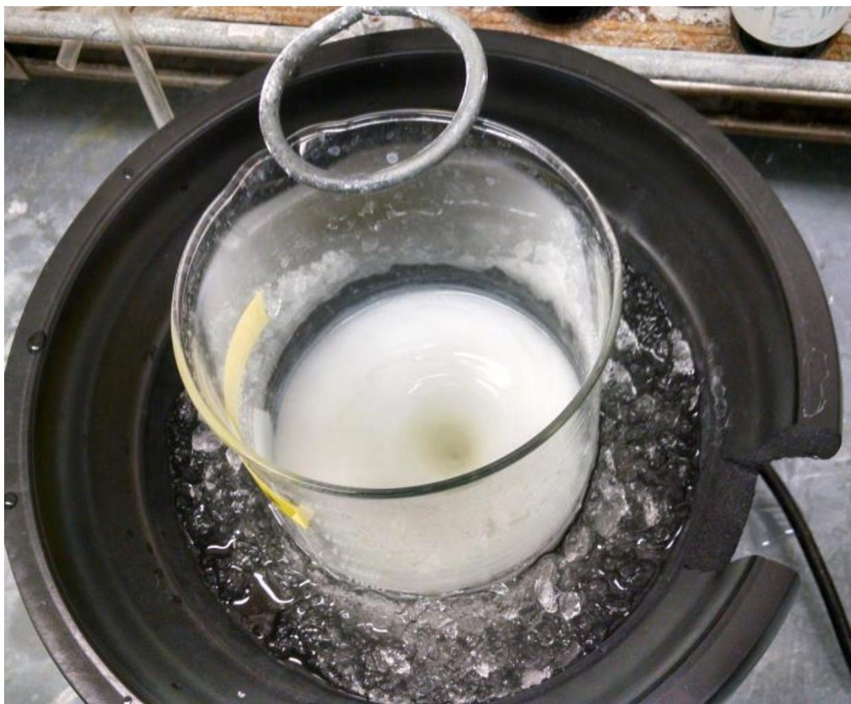
HCl salt precipitated after complete addition of 4 M HCl dioxane solution.
