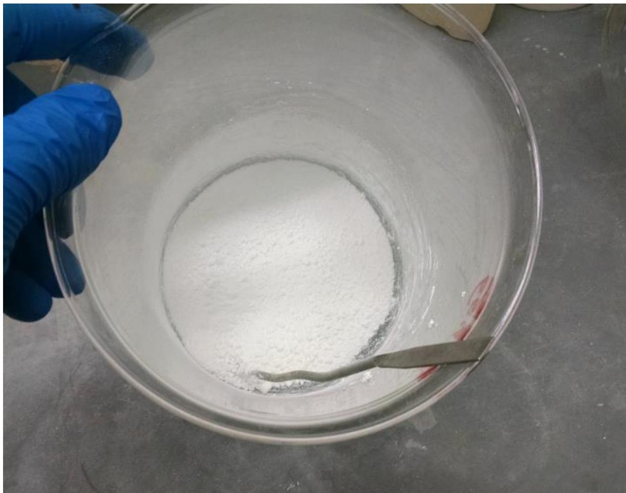
Powder of diastereomeric mixture of HCl salts prior to recrystallization (granular appearance).
