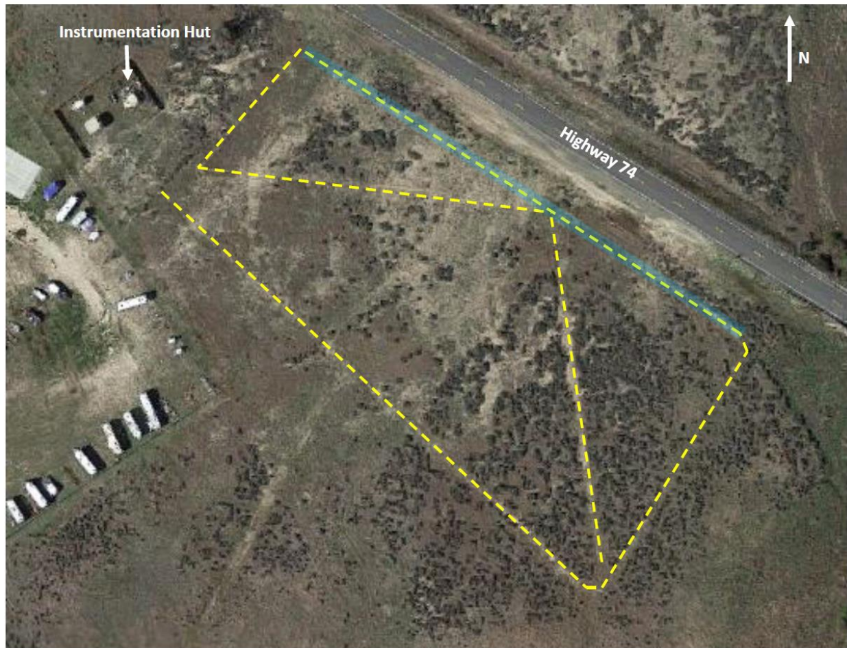
Figure 4.1: Map of the study area with cable marked with dashed yellow lines. The section of cable parallel to the road is highlighted in blue.
