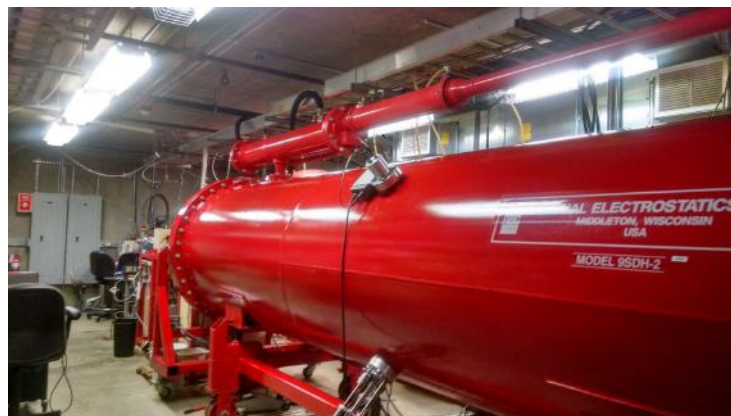
Figure 2. National Electrostatics Corporation 9SDH-2 electrostatic tandem to accelerate charged particles.
