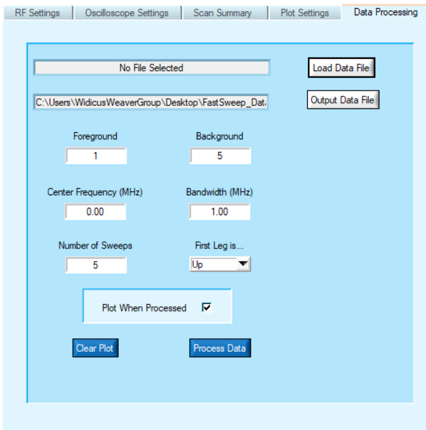
Figure 4.15: The data processing interface to provide a GUI for the Sweep.py processing script in Fast Sweep v2.0. The user is able to provide all arguments needed via a graphical user interface, including file names and paths, to process and view data within the Fast Sweep program.
