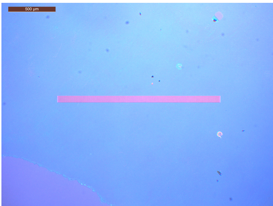
Figure 3-6: Photo displaying typical coverage of graphene transfer process on an etched test pattern. The pattern has 2 μm trenches separated by 2 μm mesas and is 1.8 mm long.
