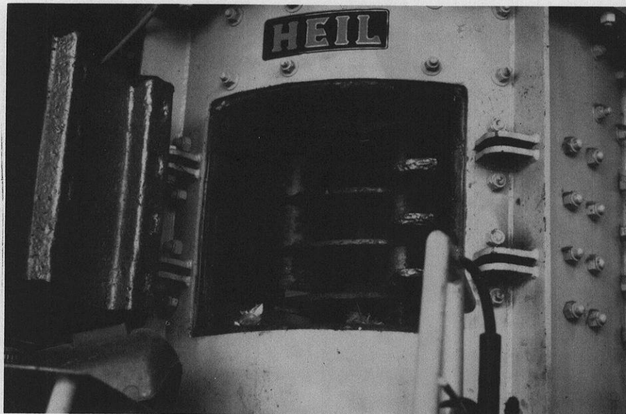
A Gondard-Tollemache hammermill located at the Madison landfill site has been used to fragment frozen tires in UW experiments.
