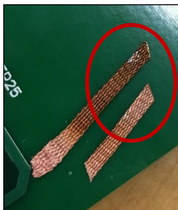
(d) Solder removed during slight die-attach degradation
