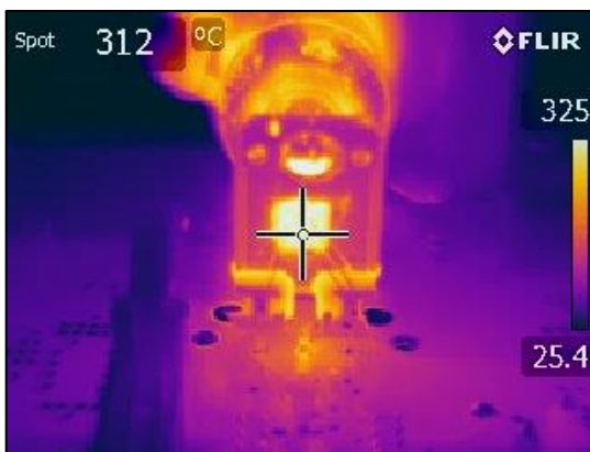
(b) Heating of the IGBT to reflow the die-attach solder
