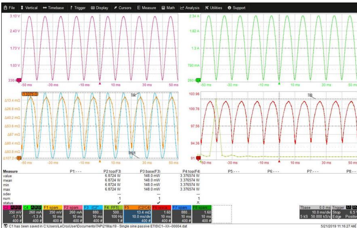
Fig. 3.2-8. Time-domain data from an ex situ ETIS experiment at f_{fund} = 100 Hz
