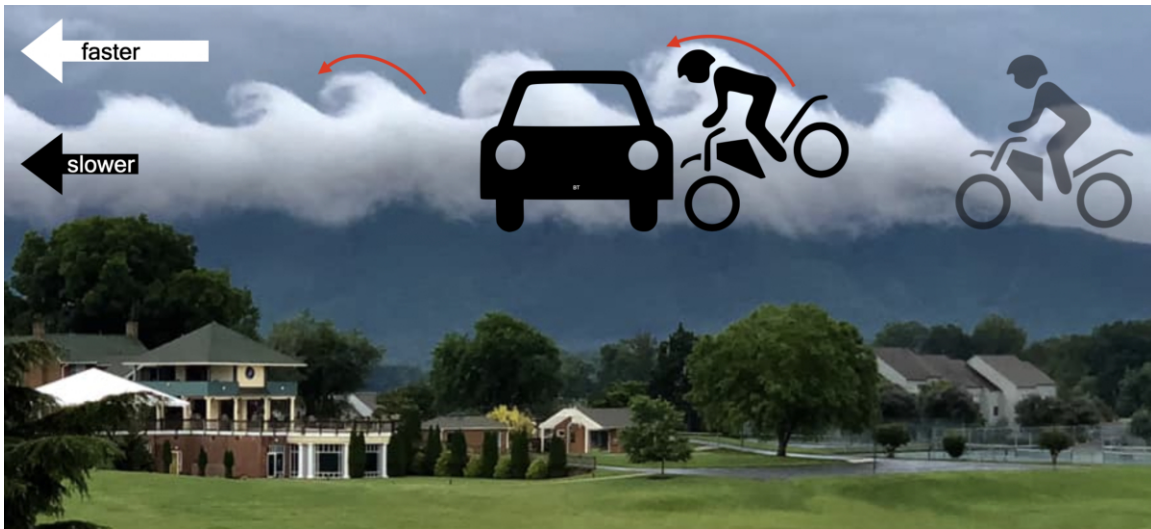
Figure 1.1: A motorcycle crashing against a car illustrates the underlying mechanism behind the Kelvin–Helmholtz instability. The instability is driven by the difference in fluid velocity. The background scene was spotted at Smith Mountain Lake, Virginia, on the evening of June 18, 2019 by Amy Christie Hunter (Facebook), which shows public excitement about the topic investigated in this thesis.
