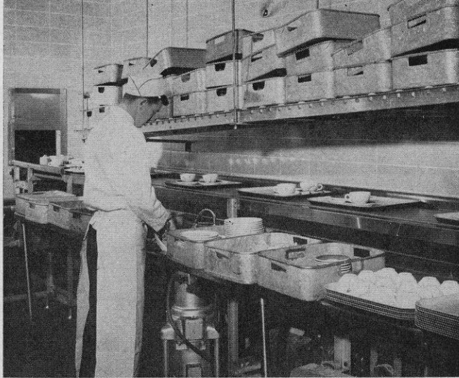
The scraping room is completely mechanized, with two conveyor belts in operation. On one patrons place empty dishes; the other takes scraped dishes to basement. Garbage, paper are ground.
