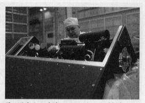
The High Speed Photometer is tested before launch.
