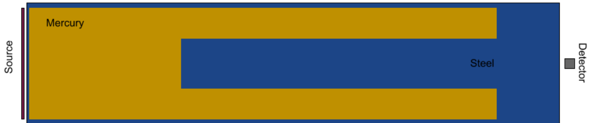
Figure 7.1: Cross-sectional view at x = 0 of test problem geometry
