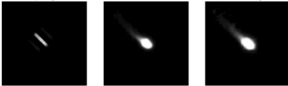
Figure 3.29: An example of melt pool prediction by machine learning. The left, middle, and right are the input, ground truth, and prediction respectively.
