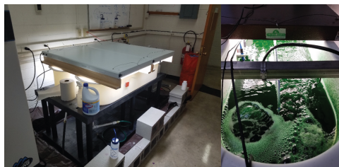
Figure 60: An image of the fully upgraded ORP system. This includes the upgraded brighter lighting that delivers light at volumetric delivery rates similar to the sun in an industrial system.
