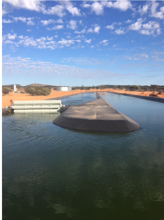
Figure 5: Figure of a large-scale open raceway pond for algal growth. Figure adapted from the MicroBio Engineering website @ https://microbioengineering.com/rw1000/
