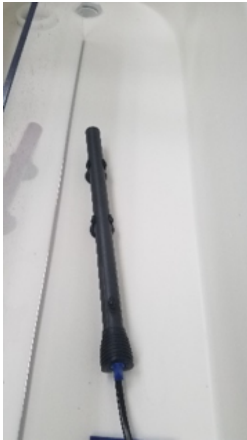
Figure 58: A 150W fishtank heater purchased to maintain temperature within the ORP.
