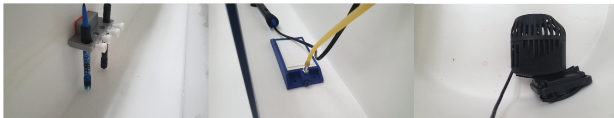
Figure 56: Left: The pH and temperature probes placed inside their magnetic probe holders. Center: Diffuser stone set on the bottom of the ORP. Right: Impeller fixed in place using magnets.
