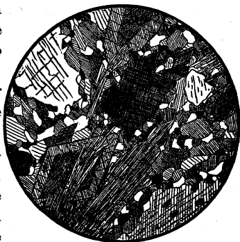
Fig. 3. Section of Hornblende-Gneiss (Metamorphosed hypersthene gabbro) from Thistle Cotton Mills, Ilchester, Md., showing peripheral granulation of feldspar, fraying out of hornblende, and development of epidote with zonal structure. X50.
