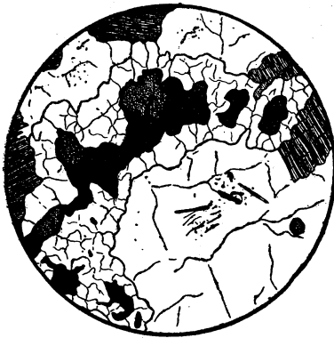
Fig. 2.—Section of gabbro-diorite from Ilchester, Md., showing ilmenite, rutile and titanomorphite. X 275.
