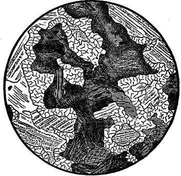
Fig. 1.—Section of gabbro-diorite from Ilchester, Md., showing reactionary rims between feldspar and hornblende. X 50.
