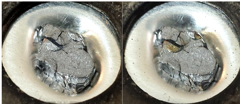
Figure 3.5: 99.999% pure chromium metal pressed in to a silver disc before (left) and after (right) irradiation with 40 \mu\text{A} for one hour with direct jet water cooling on the rear target face.
