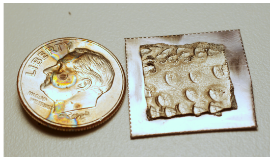
Figure 7.2: Spot welded ^{nat}\text{Y} to Ta. Welds were conducted in a raster pattern across the target face.
